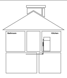
Your new *Aqua-Pure* Water Filter installs on the cold water line feeding the ice-maker. Complete installation instructions included for your convenience.
